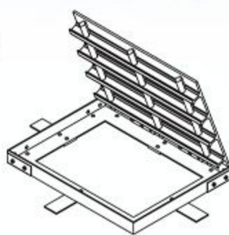
FRP CHEQUERED PLATE Grating C/W FRP Frame
